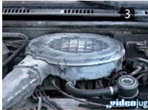
Fig : Cleaning of air filter housing
