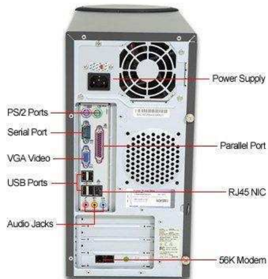
Figure 2: CPU Cabinet Back Panel
