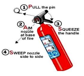
**Step 3: Squeeze** or Press the handle together. This will release the extinguishing agent.
